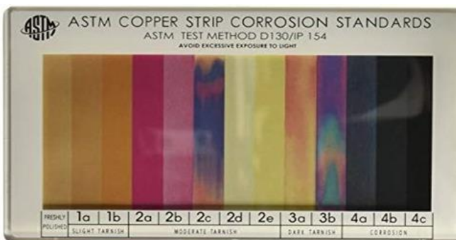
Fig. 11. Copper strip corrosion standard result of Diethyl Ether Diesel Blends.
