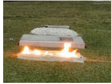
Fig 6: PHIZ test on sand [2]
