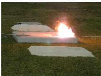
Fig 5: PHIZ test on Concrete [2]
